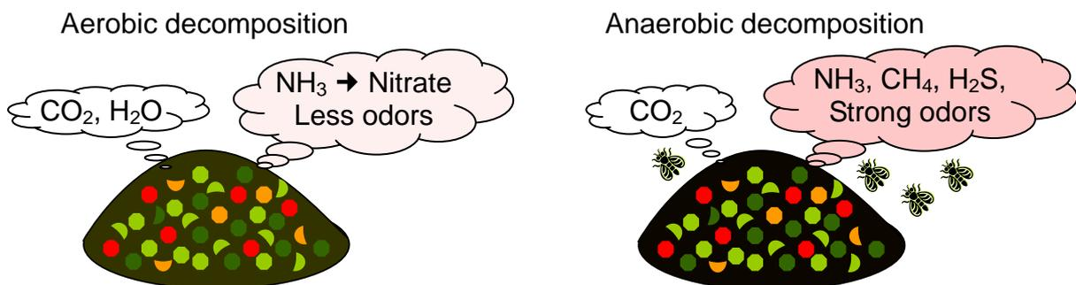
Comparison aerobic decomposition and anaerobic decomposition
