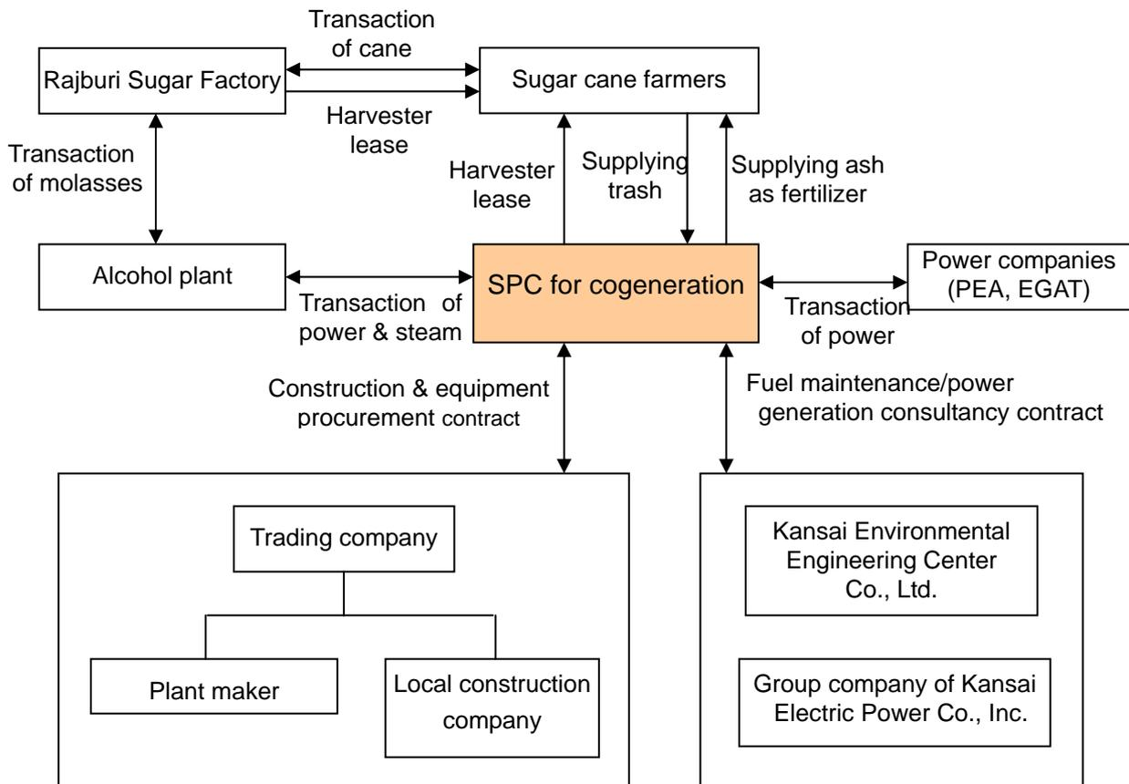
Figure 5. Implementation structure of the project (draft).
